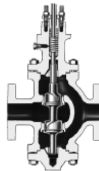
REVERSE-ACTING DOUBLE-PORTED GLOBE-STYLE VALVE BODY
