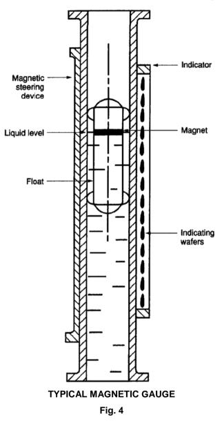
**Precautions**: Magnetic gauges must not be used in areas where forces or matter will affect the magnetic fields. This includes areas that contain items such as steel support straps, heater wires, and steam-tracing tubing.
