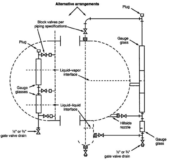
GAUGE GLASS MOUNTING ARRANGEMENT FOR HORIZONTAL VESSELS AND FOR INTERFACE MEASUREMENT
