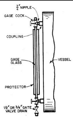
TUBULAR GAUGE GLASS CONNECTIONS TO VESSELS
